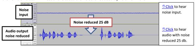
High tier radios now feature noise cancellation for more improved audio quality in noisy environments. Noise cancellation uses more than one microphone in the transmitter to distinguish noise sources from speech. This allows for noise to be cancelled, thus improving the signal-to-noise ratio for the radio user. This is not a part of the vocoder technology, but it does apply to improve the audio quality in many public safety and private LMR applications.
