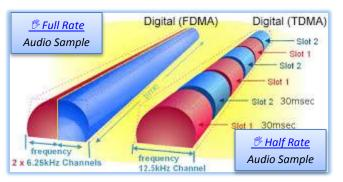
radio bands. Newer properly equipped radios can operate in either FDMA or TDMA modes in order to interoperate with older radios that are only capable of FDMA. The standard [1] also includes a parametric conversion feature to convert full rate audio to half rate, or vice versa. This allows infrastructure equipment to route audio between FDMA channels and TDMA channels without reverting back to
